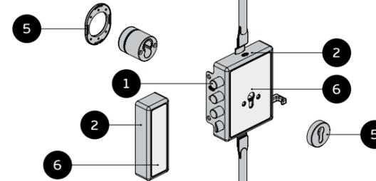
**6. Stainless steel custom covers with different colors and finishes. Powder coating with colors available in White and Gray. PVD TITANIUM finish in Black, Gold, Copper and Chocolate. / Caixa em aço com tampas personalizadas com diferentes cores e acabamentos. Lacado em Branco e Cinza. Acabamento PVD TITANIUM Black, Gold, Copper e Chocolate.**
