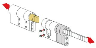
5. Insert the same size of spacer piece and brass tube to make the adjustable cylinder match the old cylinder.
