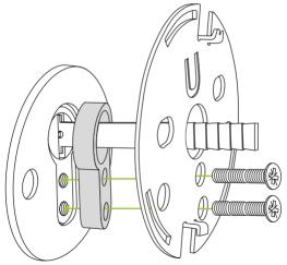
IMPORTANT! Make sure that the lock still works! Make sure that the lock still works properly by turning the tailpiece. If you can't lock and unlock this way please loosen the cylinder screws. (b)
