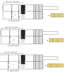
6. Assemble the cylinder and screw the small screws back in on both sides of the cylinder.
