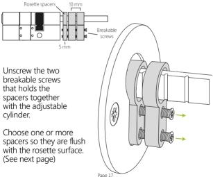
IMPORTANT! Avoid pulling the cylinder out of place. It is important that the spacer is flush with or sticks out from the hole in the rosette plate.
