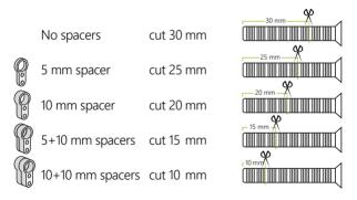
Use a wirecutter, two pliers or bend the screws forth and back several times in a vice to break them.
