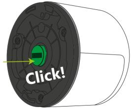
**13.** Fit the tailpiece to the middle of the housing base Fit the Danalock over the back plate. Make sure the tailpiece hits the slide in the middle of the adaptor.
