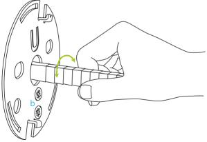
11. Give the tailpiece the right length To avoid damaging the Danalock you will have to shorten the new cylinder tailpiece to **max. 35 mm** from the door surface. Use two pliers or a wire cutter to shorten the tailpiece.
