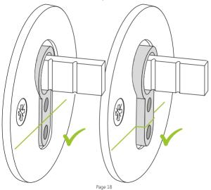
9. Break the screws to the right length Depending on which spacer or spacer combination you chose, it is now important that the screws that fasten the cylinder to the back plate have the right length. Use this chart to find the right length:
